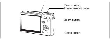
The simplest procedure for taking still pictures is described below. The flash fires automatically depending on the light conditions.
